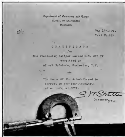
FIG. 47—Special Micrometer Caliper and reduced fac-simile of U. S. Bureau of Standards certificate.
